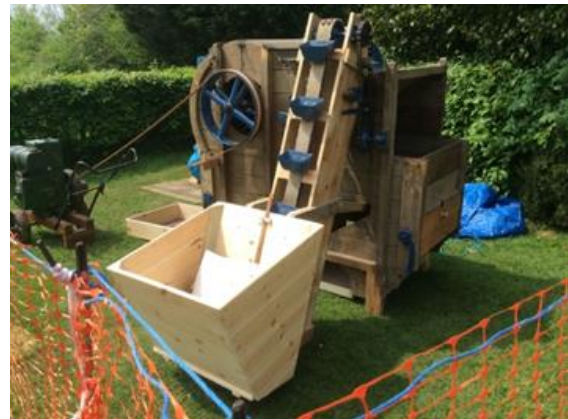
Our recently restored 19 th century winnower, belt driven from a small standing engine
