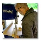
A special sliding jig was used to allow the wedges to be cut, each accurate to within just 1 mm.
